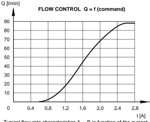
Typical flow rate characteristics  $A \rightarrow B$  in function of the current supplied to the solenoid (D12 version, max current 2.8 A, PWM 100 Hz).
