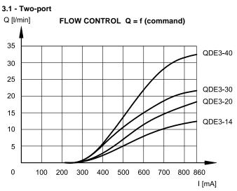
Typical flow rate characteristics  $A \rightarrow B$  for controlled flow rate: 14 - 20 - 30 - 40 l/min in function of the current supplied to the solenoid (D24 version, maximum current 860 mA, PWM 100 Hz)
