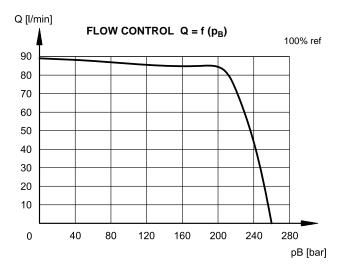
Pressure drops with flow  $A \rightarrow P$ . Obtained with  $Q_B = 0$  (no current)
